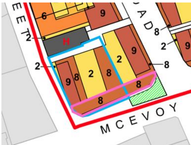
Figure 32: DCP map with the site outlined in blue and 8 storey southern street wall outlined in pink
