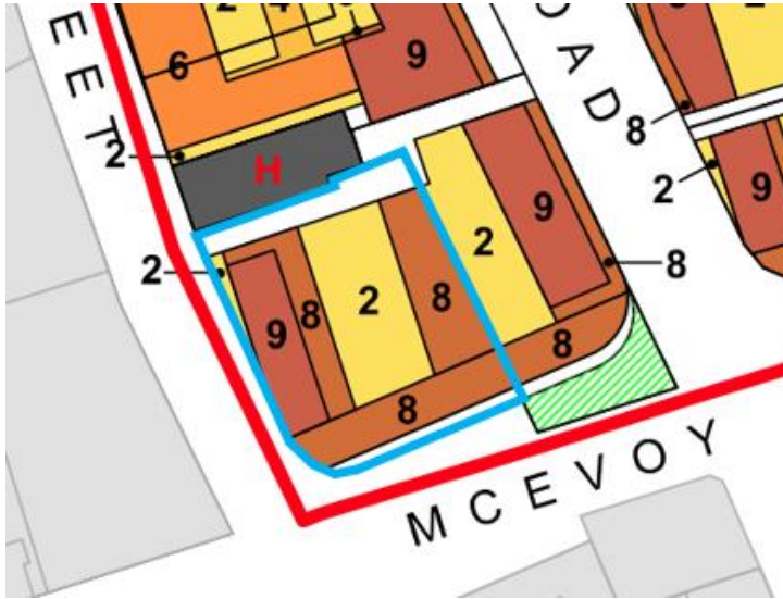
Figure 27: Height in storeys for residential development permitted under the SDCP 2012, with the site outlined in blue
